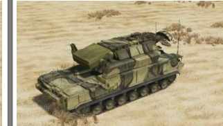
SA-15 Gauntlet Radar Range: 13.0nm RWR ID: 15 HARM Code: 119 Max Rg: 6.5nm Max Alt: 26,000ft
