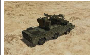
SA-8 Gecko TEL Radar Range: 16nm RWR ID: 8 HARM Code: 117 Max Rg: 8.0nm Max Alt: 21,000 ft
